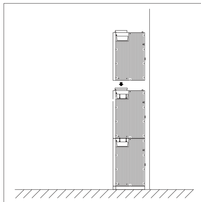
Step 2: Stack the batteries in sequence, tighten the handlebar screws on both sides of the batteries.
