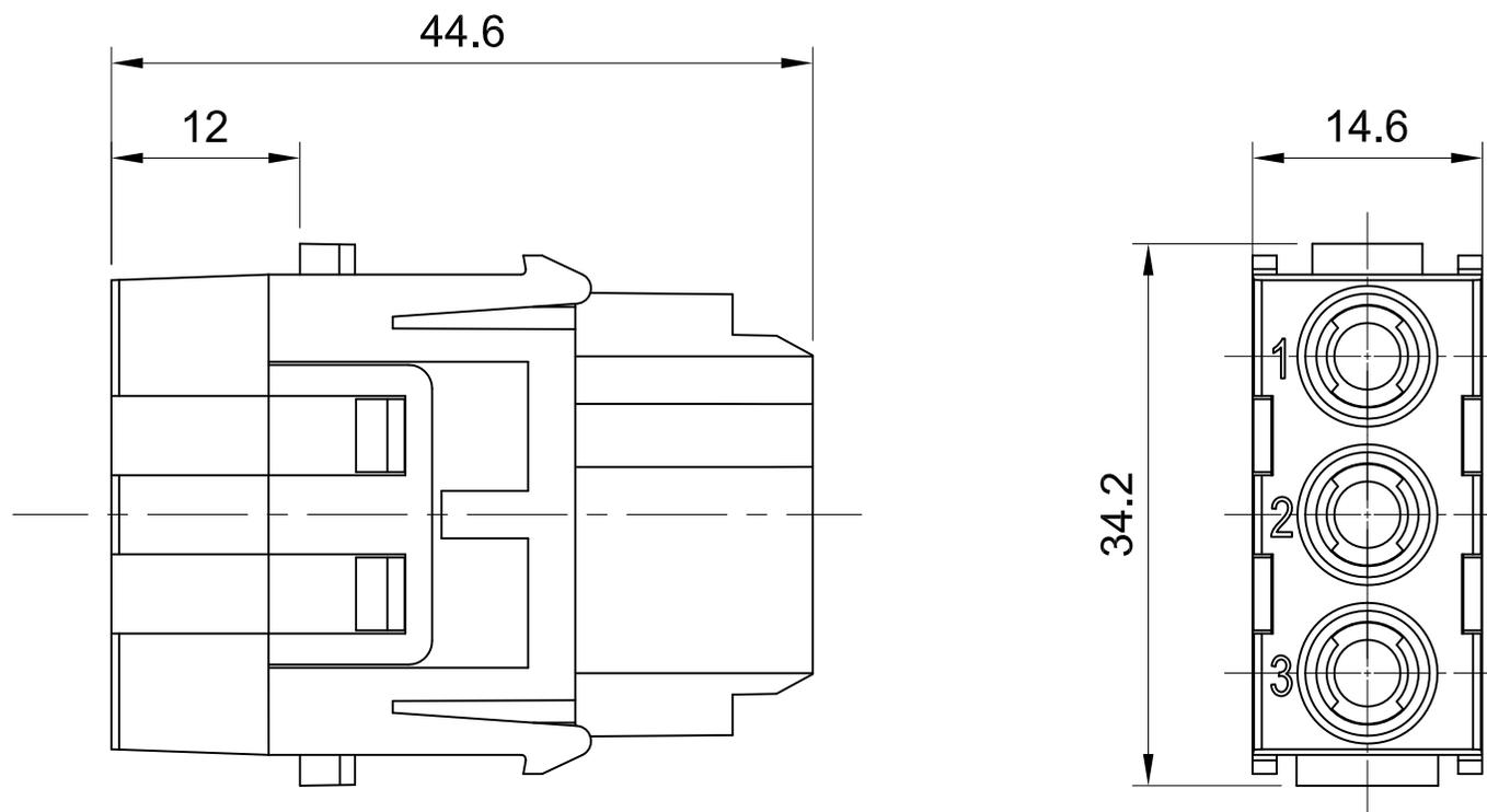
Wire diameter over insulation  $\leq 4.8\text{mm}$  stripping length 9.5mm
